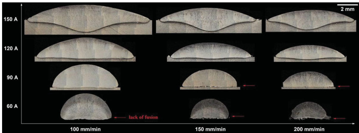
Figure 43 - Optical microscopies of the single-track cross-sections
