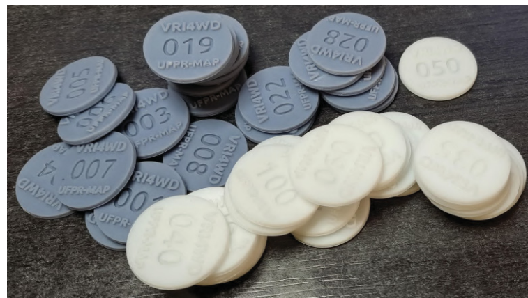
Figura 6.7: Tags manufacturing in a printer, liquid resin. Showing the name of the dataset and the position number on the map. Tags with a diameter of 30 mm and a thickness of 2 mm, using a projection for the letters and a recess for the number. Used in two colors, gray or white, to differentiate multiples of 5 from white tags.
