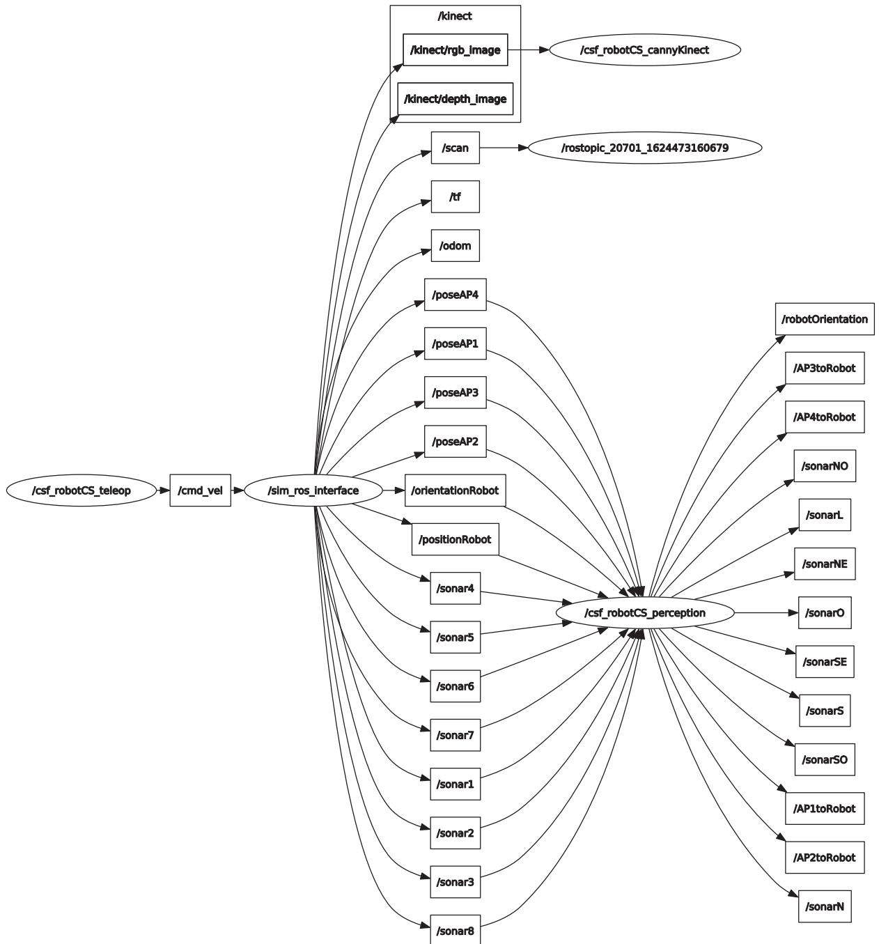
Figura 5.8: Displaying graphs of running ROS nodes (ellipses) with connecting topics (rectangles) and packages (obtained by the tool rqt_graph ). The ROS nodes running robot teleoperation /csf_robotCS_teleop , interface ROS with CoppeliaSim /sim_ros_interface , edge detection algorithm and OpenCV function with Kinect /csf_robotCS_cannyKinect , and preprocessing sensor information /csf_robotCS_perception .
