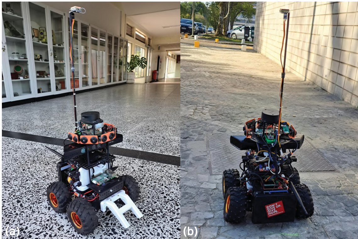
Figura 5.14: VRI4WD Mobile Robot Platform. The mechanical platform is a 4WD all-terrain chassis. (a) The Figure shows the robot moving along the trajectory in an indoor environment. (b) The Figure shows the robot moving along the trajectory in an outdoor environment.
