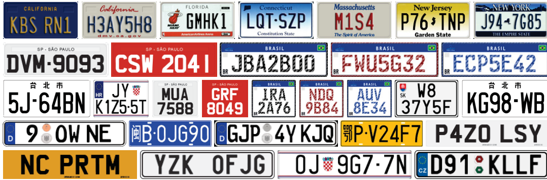
Figure 7.1: Examples of the template-based LP images we created for this study. Notably, any sequence can be generated for each template. The background and character images were manually gathered from the internet 19 . During training, these LP images are subjected to various transformations to introduce variability.
