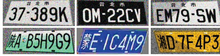
Figure 8.4: Some of the many LP images we created to mitigate overfitting. The images in the top row simulate LPs from vehicles registered in the Taiwan region (as in AOLP), while those in the bottom row simulate LPs from vehicles registered in mainland China (as in CCPD).
