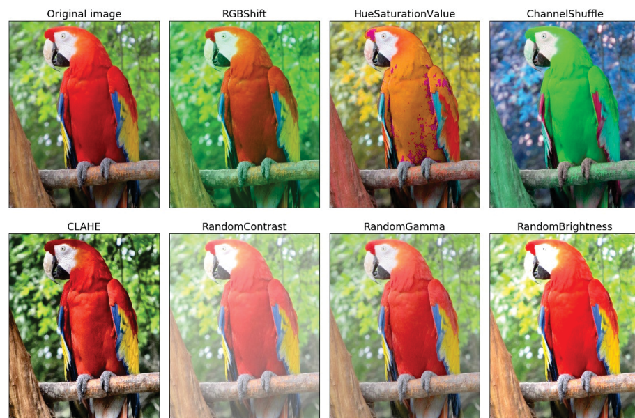
Figure 2.21: An example of how some augmentations can be applied to create new images from the original one. Image reproduced from https://github.com/albumentations-team/albumentations/ .
