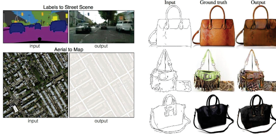
Figure 2.18: Image-to-image translation is a concept introduced by Isola et al. (2017) that encompasses many kinds of transformations of an image: converting segmentation masks into images, converting aerial photos into maps, converting sketches into photorealistic images, among others. Image adapted from (Isola et al., 2017).
