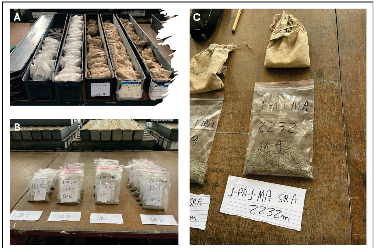
Figure 33 – Photomosaic of sample selection for compositional kinetic analysis. A) Box with cuttings of Pimenteiras formation at the well 1- PA-1-MA; B) set of samples selected inside of each organic rich interval of the Pimenteiras fm. (A, B, C and D); C) detail of the selected sample at level A of the Pimenteiras formation, one of the selected samples for kinetic study.
