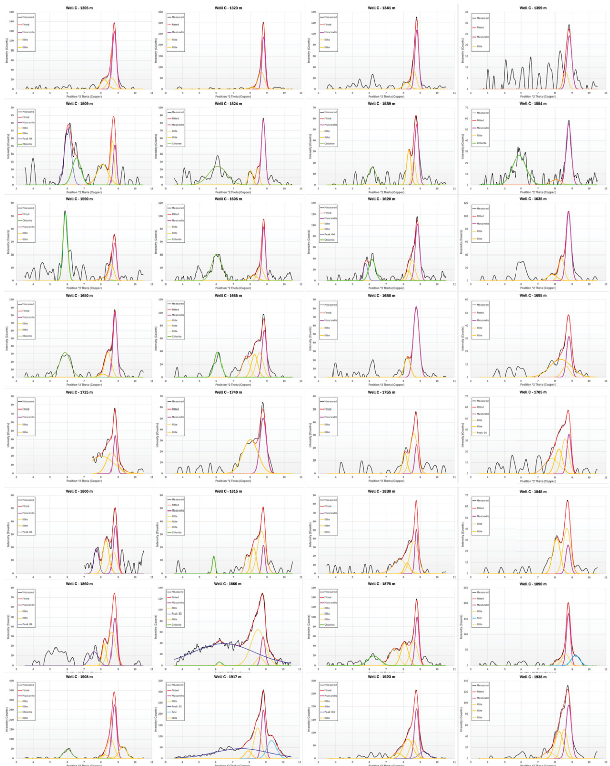
XRD Decomposition chart of the Well C (depths from 1305m to 1938m), with interpretation, showing the measured XRD profile (black), the interpreted clay mineral phases (orange=Illite; pink=Muscovite; light green=Chlorite; blue=Pyrophyllite/Talc) and the fitted profile (red).
