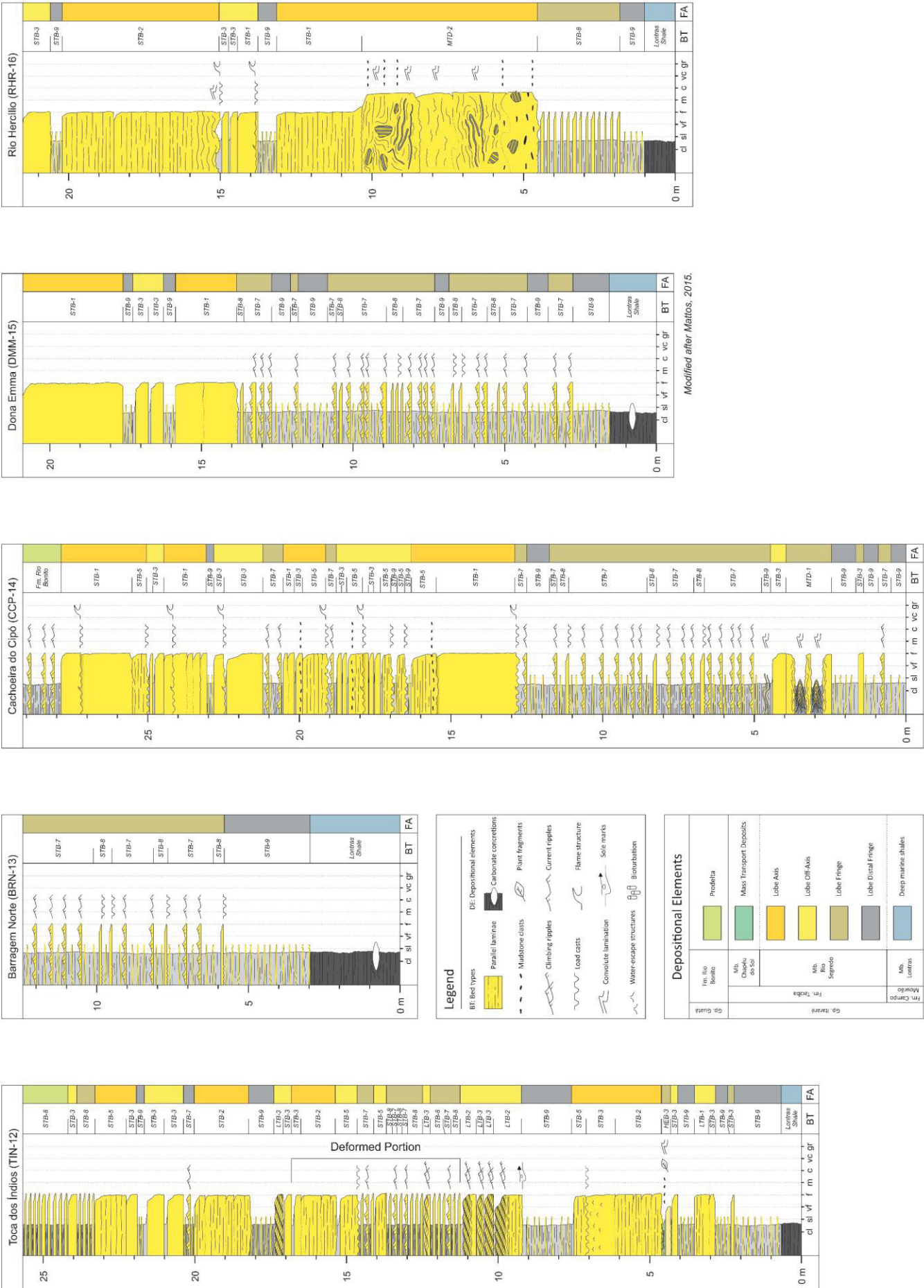
Figura 27. Sedimentary logs with graphical representations of bed types and facies associations. Logs TIN-12, BRN-13, CCP-14, DMM-15, RHR-16.
