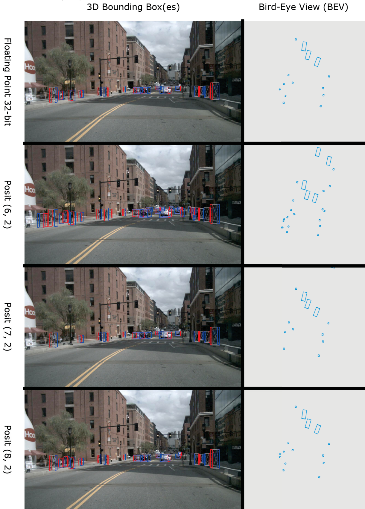
FIGURE 30 – 3D BOUNDING BOXES AND BIRD-EYE VIEWS OBTAINED FROM THE QUANTIZATION OF BOTH REGRESSION HEADS, USING POSIT-AS-STORAGE (PAS).
