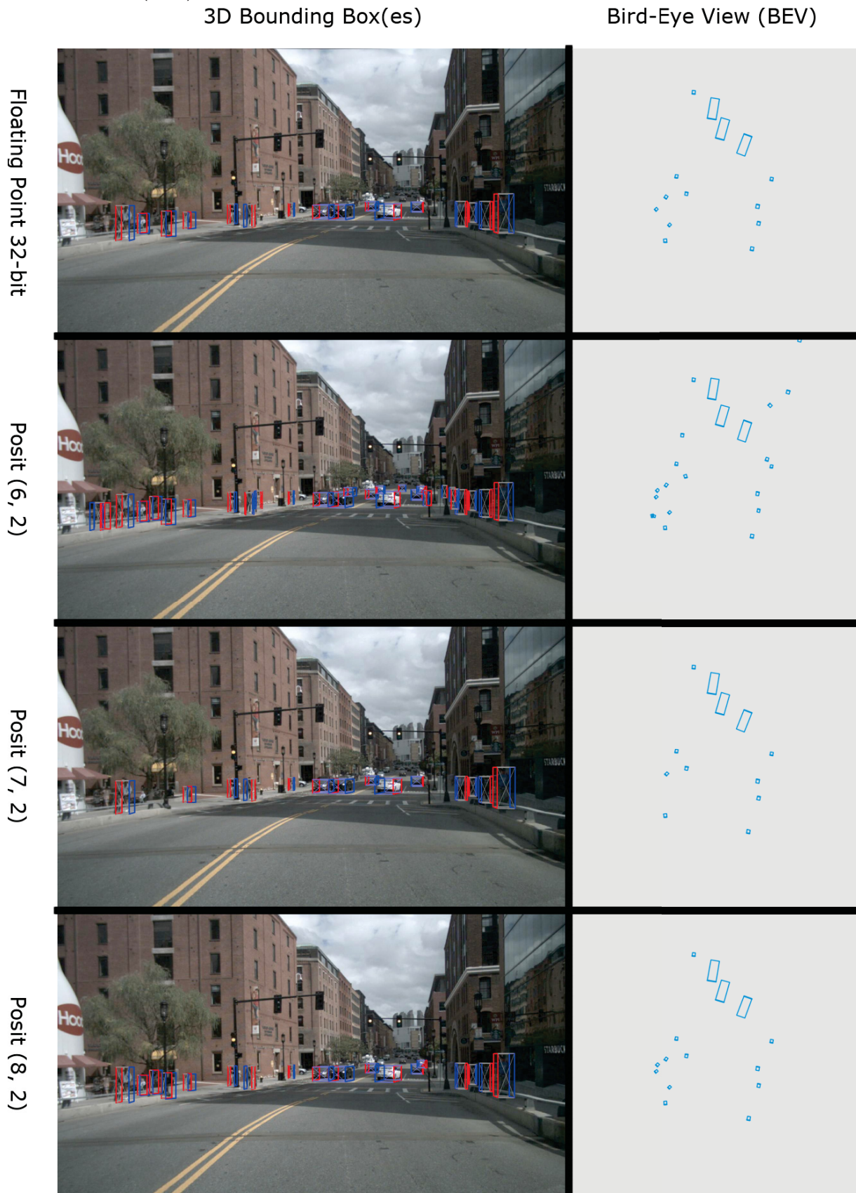
FIGURE 33 – 3D BOUNDING BOXES AND BIRD-EYE VIEWS OBTAINED FROM THE QUANTIZATION OF PRIMARY REGRESSION HEADS, USING POSIT-AS-STORAGE (PAS).
