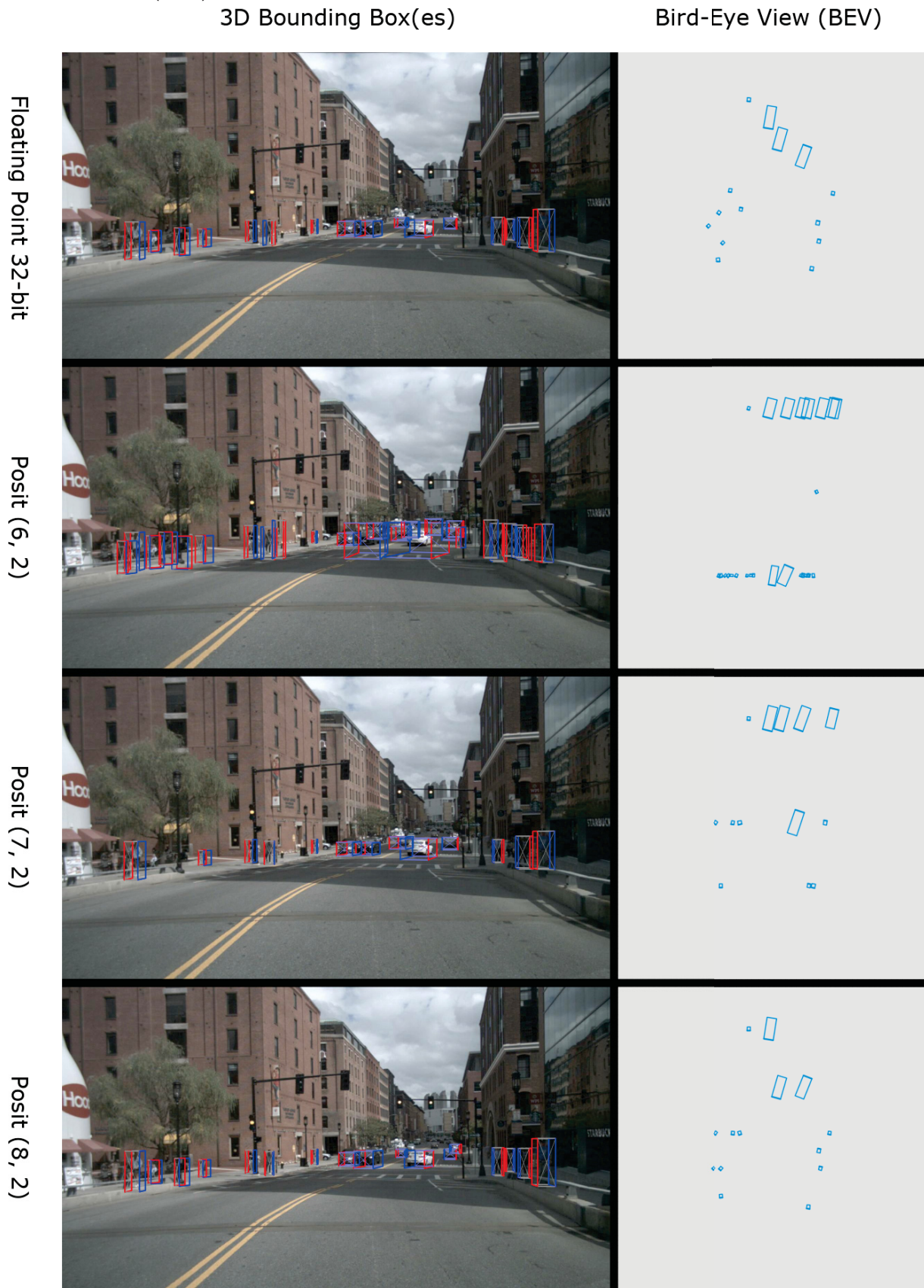
FIGURE 41 – 3D BOUNDING BOXES AND BIRD-EYE VIEWS OBTAINED FROM THE QUANTIZATION OF BOTH REGRESSION HEADS, USING POSIT-AS-ARITHMETIC (PAA).
