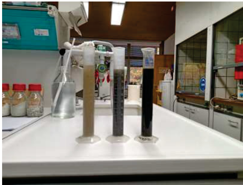
Figure 56 – Output samples for feeding flow rates of 300, 200, and 150 L/h on November 1 st .
