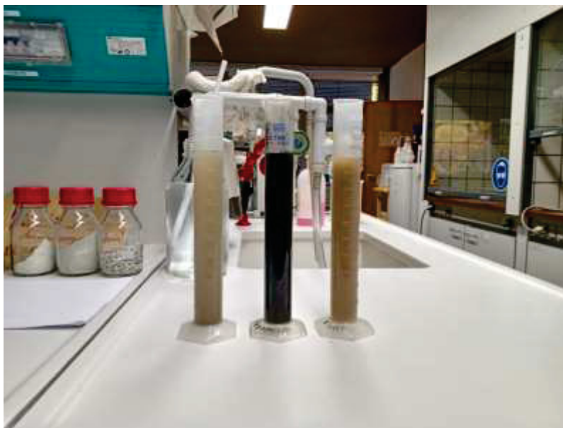
Figure 14 – Example of feeding mixture (right), substrate (middle), and output (left) collected on November 1st.
