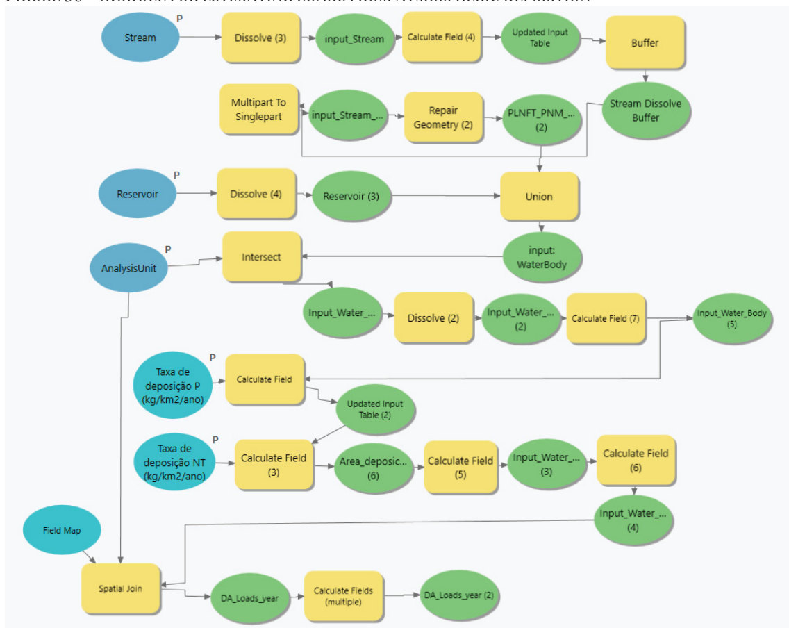
FIGURE 36 – MODULE FOR ESTIMATING LOADS FROM ATMOSPHERIC DEPOSITION
