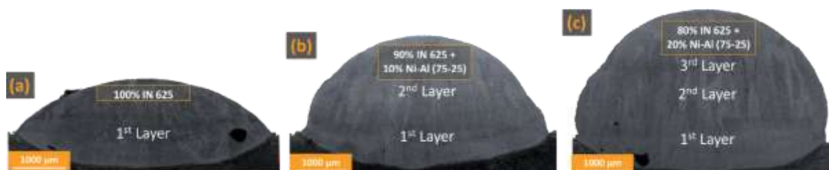
Fig. 2. PTA-AM micrographs showing the buildup layers and their compositions: (a) first layer with 100% IN 625; (b) second layer with 90% In 625 and 10% Ni-Al; and (c) third layer with 80% IN 625 and 20% Ni-Al.
