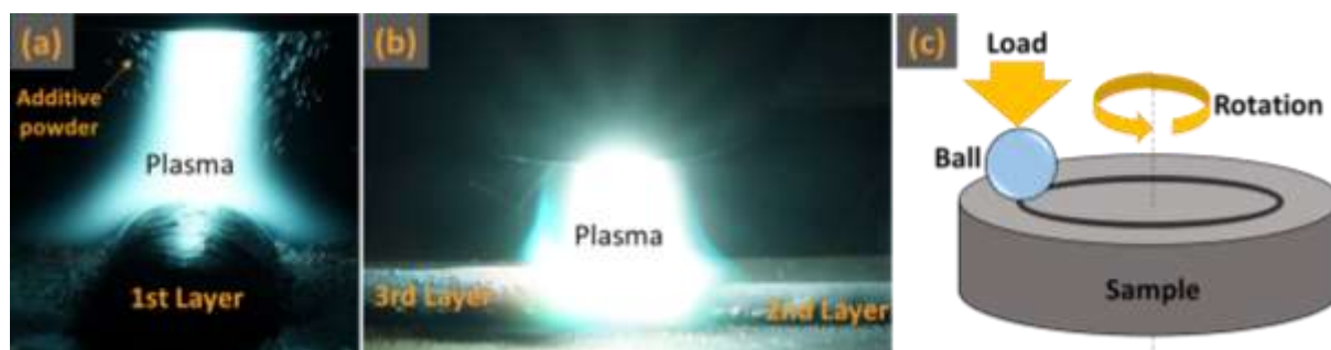
Fig 1. PTA-AM photograph showing (a) the plasma torch in transverse direction and (b) the deposition sequence for second and third layers in longitudinal direction. (c) Schematic drawing of the wear test.
