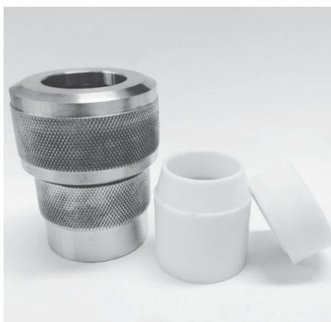
FIGURA 13. REATOR DE TEFLON<sup>®</sup> COM CAMISA DE AÇO INOXIDÁVEL
