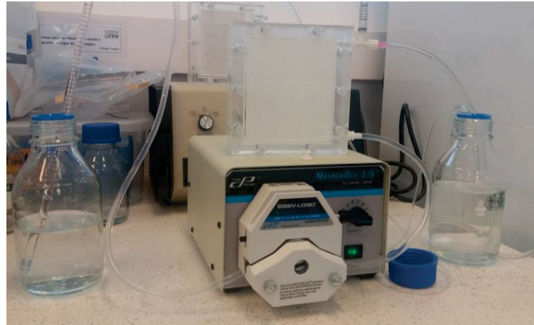
Membrane filtration system.
