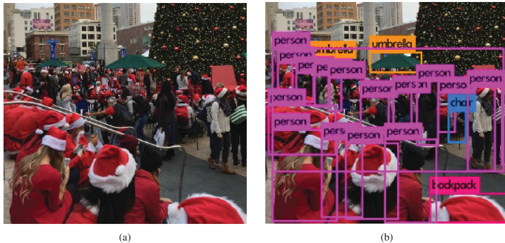
Figure 2.11: Illustration of one of YOLO’s limitations, where detection can miss objects that are too close. In (a), there are 9 individuals in the lower left corner, but only 5 were detected, as can be seen in (b). Replicated image from (Redmon et al., 2016a).
