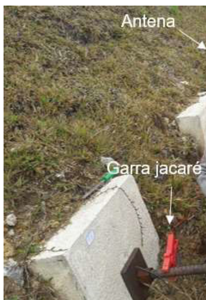
Figura 3.52 – Ensaio Reflectometric Impulse Measurement Technique
