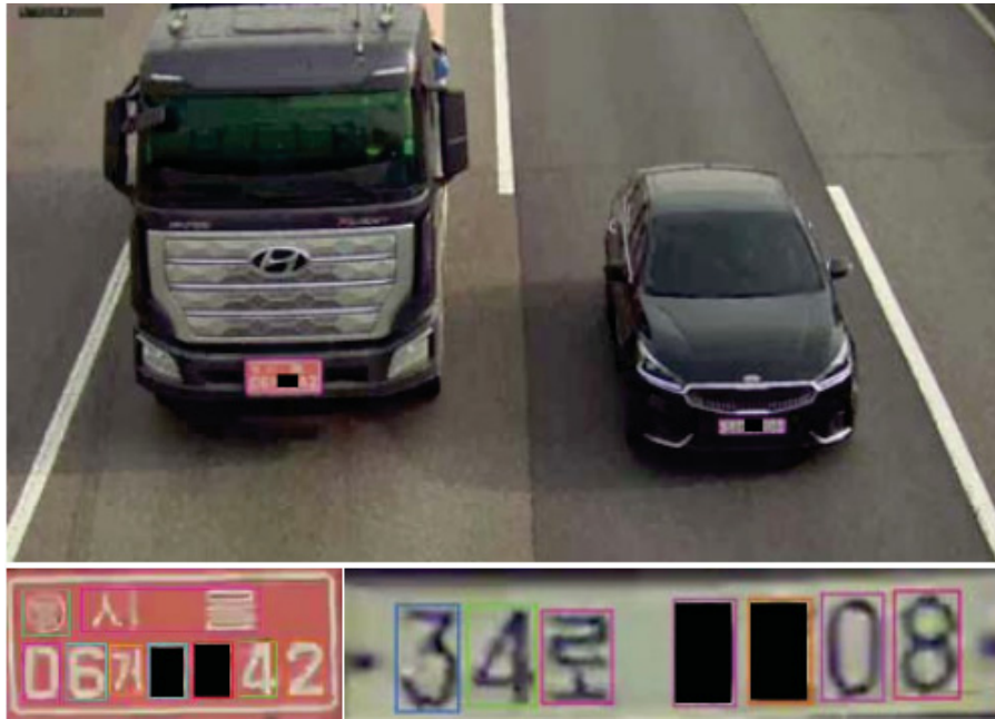
Figure 3: Demonstration of the YOLOv4 algorithm detecting different individual details of a license plate alongside a license plate for multiple objects – [2].
