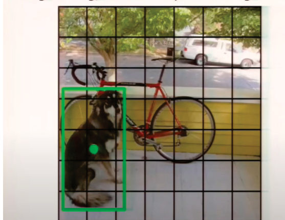
Figure 92: Representation of the attribution of the dog class to the specific cell using a centered x,y position. The box central position is going to define the class attributed to each cell on the grid.
