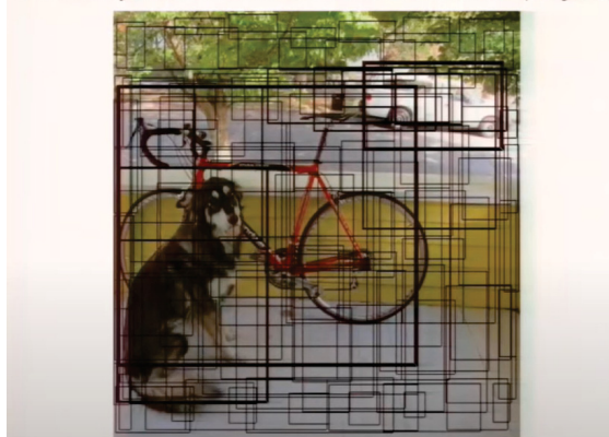
Figure 86: At the end of the process, many different bounding boxes are present in the picture – predicting different possible objects.
