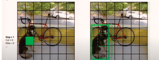
Figure 94: Out of all the bounding boxes falling with the (x,y) coordinates to that specific cell, the best one is chosen and then adjusted – increasing the total confidence of the bounding box.
