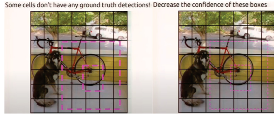
Figure 95: Some of the bounding boxes is a specific location doesn't have an object in that area, so the level of confidence in that region is reduced.
