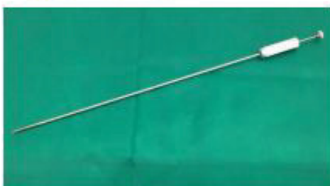
Figure 3. Toggle applicator produced in stainless steel. Leaked tube with cutout at the tip for wire fitting, 0.5mm wall thickness, 50cm long and 5mm in diameter. Inside is another stainless steel cylinder with 3.5mm to push the "toggle".
