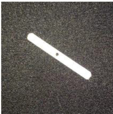
Figure 2. Toggle - Polyamide lever 2cm long, 3.2mm wide and 1.5mm thick.
