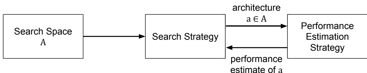
Figure 3.1: Abstract illustration of Neural Architecture Search methods. Adapted from [30].
