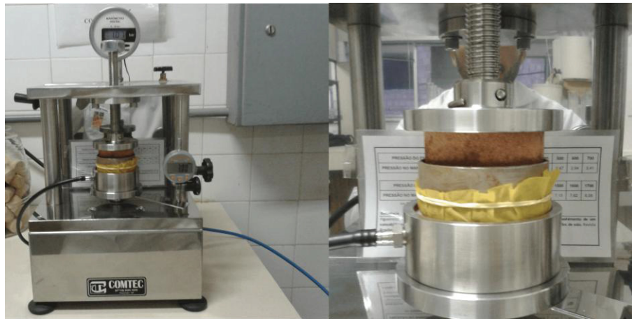
Figure 3: Compression apparatus used in the uniaxial compression test
