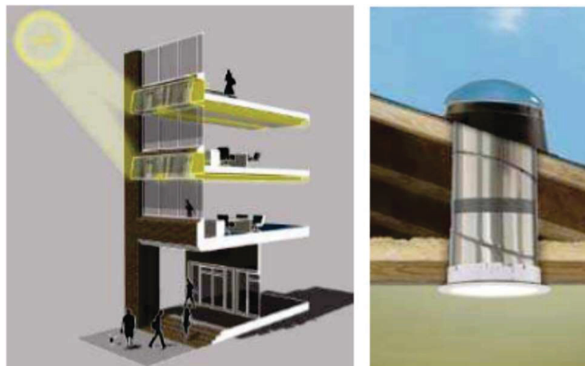
FIGURE 7 – LIGHT DUCT EXAMPLE
