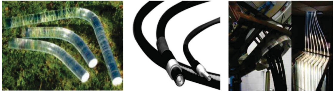
FIGURE 6 – TOTAL REFLECTION CONDUCTORS EXAMPLES: SOLID GUIDES (LEFT), LIQUID GUIDES (MIDDLE) AND OPTIC FIBER (RIGHT)
