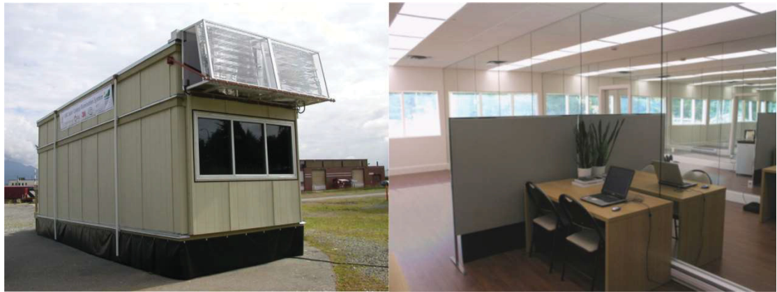
FIGURE 8 – TEST FACILITY WITH SOLAR CANOPY MOUNTED ABOVE THE SOUTH WALL WINDOW (LEFT) AND INTERNAL VIEW ILLUMINATED BY THE DAYLIGHTING SYSTEM (RIGHT)
