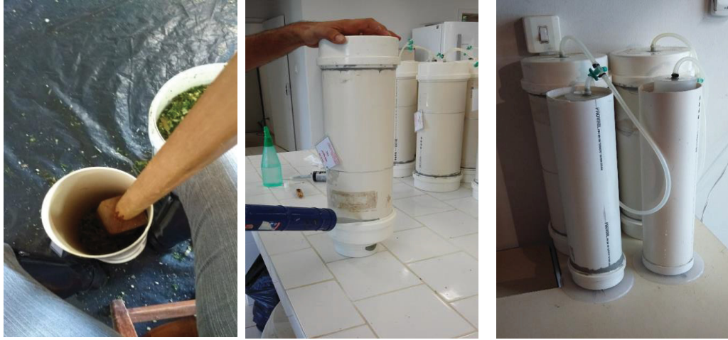
FIGURE 8. PVC silos filled with chopped maize forage, closed with a proper lid, sealed adhesive plastic polymer and equipped with an apparatus to measure gas production.
