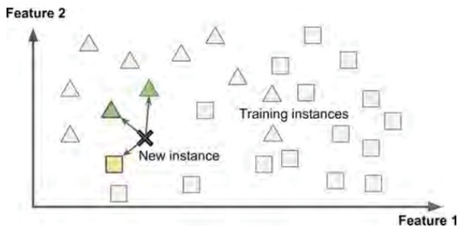
Figure 2.7: Example of the KNN algorithm, in which two features (feature 1 and feature 2) are used to discriminate triangles and squares, 3 nearest training instances from X are found through euclidean distance, in this case X is considered a triangle. Source: (Géron, 2019)
