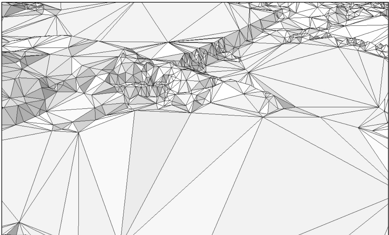
FIGURA 2.5 - GRADE IRREGULAR TRIANGULAR (TIN)
