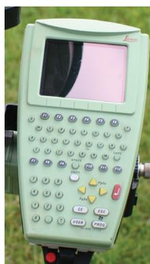
FIGURA 44 – GPS *LEICA* RX1250
