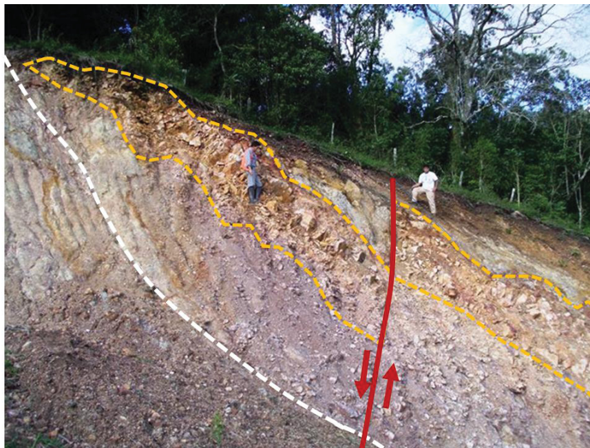
Figure 1 - SW to NE (Left edge in the photo) cross-cutting view of Torre Orebody. The dashed yellow line surrounds the main massive quartz-chalcedony vein, which is the richest portion (up to 1.2g/t Au). The white dashed line limits the stockwork and veinlet mineralization zones at the edges of the main central lode. All rocks are cutting by younger normal fault, not mineralized, with E-W direction and subvertical dipping.
