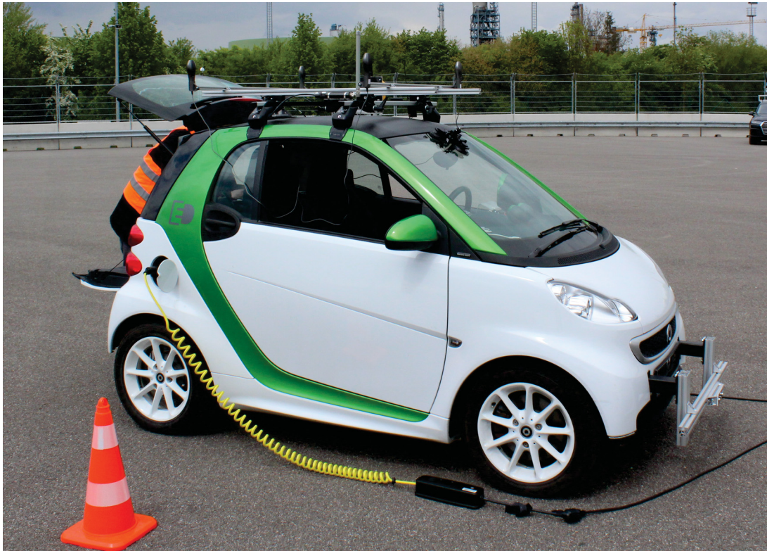
Figure 32: Smart Electronic Drive set up with the microphone array mount.
