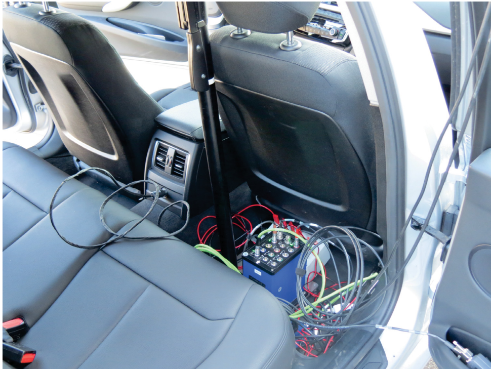
Figure 35: ADMA module installed in the police vehicle.
