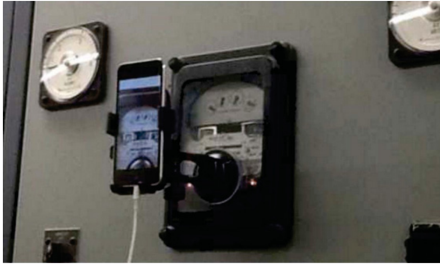
Figure 3.7: Images were captured every 15 minutes and send wirelessly to a remote server. Extracted from Tang et al. (2015).
