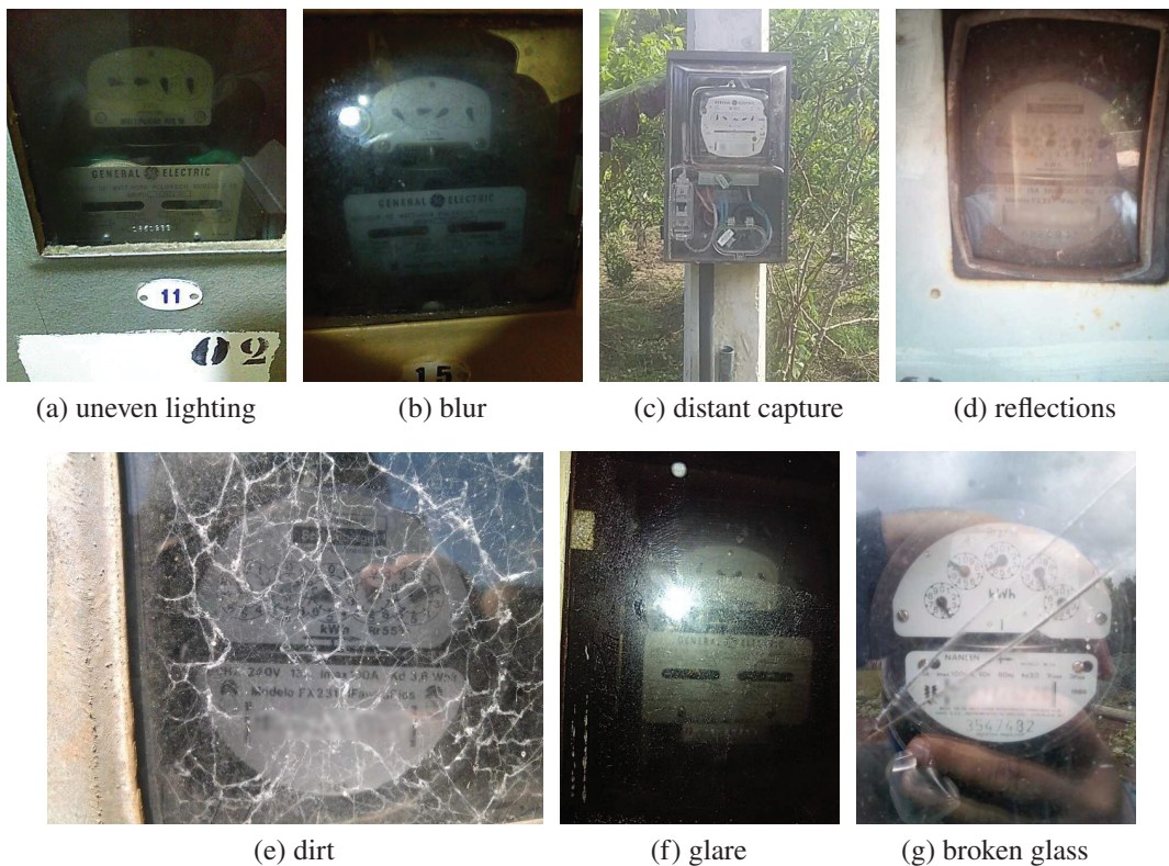
Figure 4.6: Samples of the challenging scenarios present on the provided images. We selected for the UFPR-ADMR-v2 dataset 5,000 images in which it was possible for a human to recognize the correct reading of the meter. Note that most of the dials presented above are not readable, and were not selected for the dataset. We blurred the region containing the consumer unit number in each image due to privacy constraints. None of the images above were selected to our database, they are displayed solely for illustration purposes.
