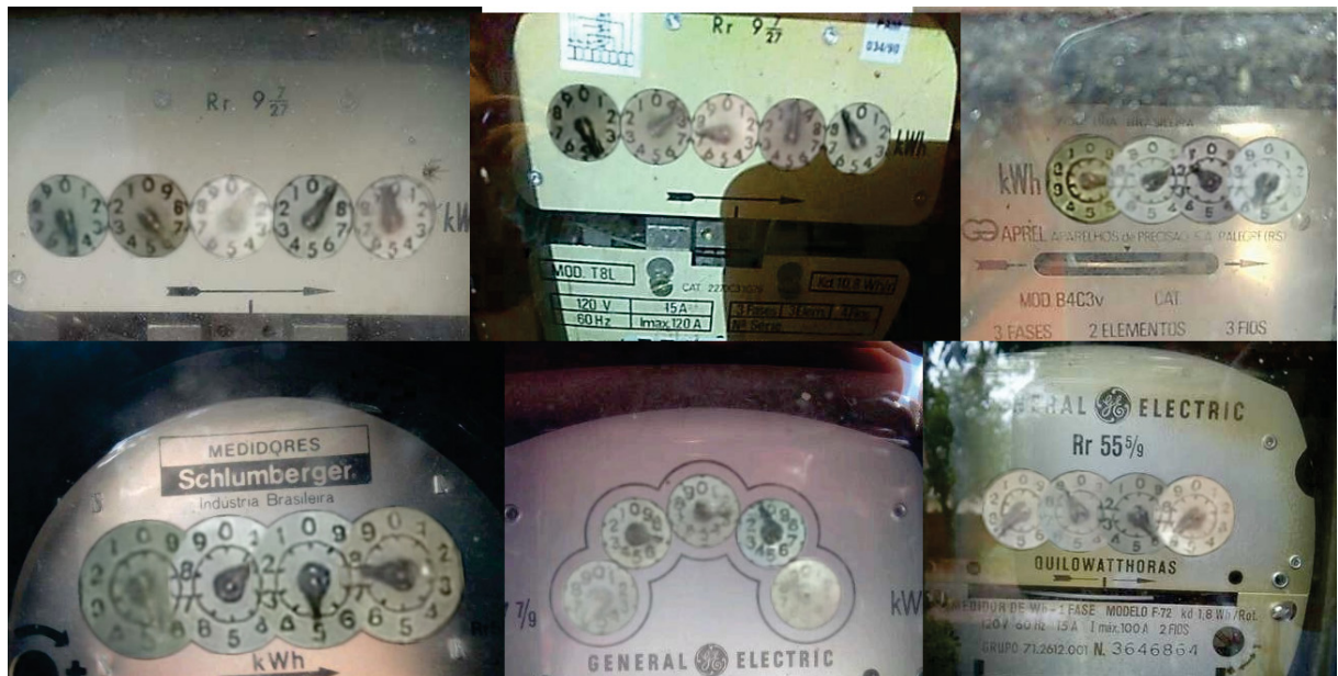
Figure 6.4: Samples of the 50,000 generated images. After generating the individual dials, using the annotated mask and bounding rectangle, we correct the perspective and insert the synthetic dials in the original image. Afterwards, the image is warped back into the original perspective.
