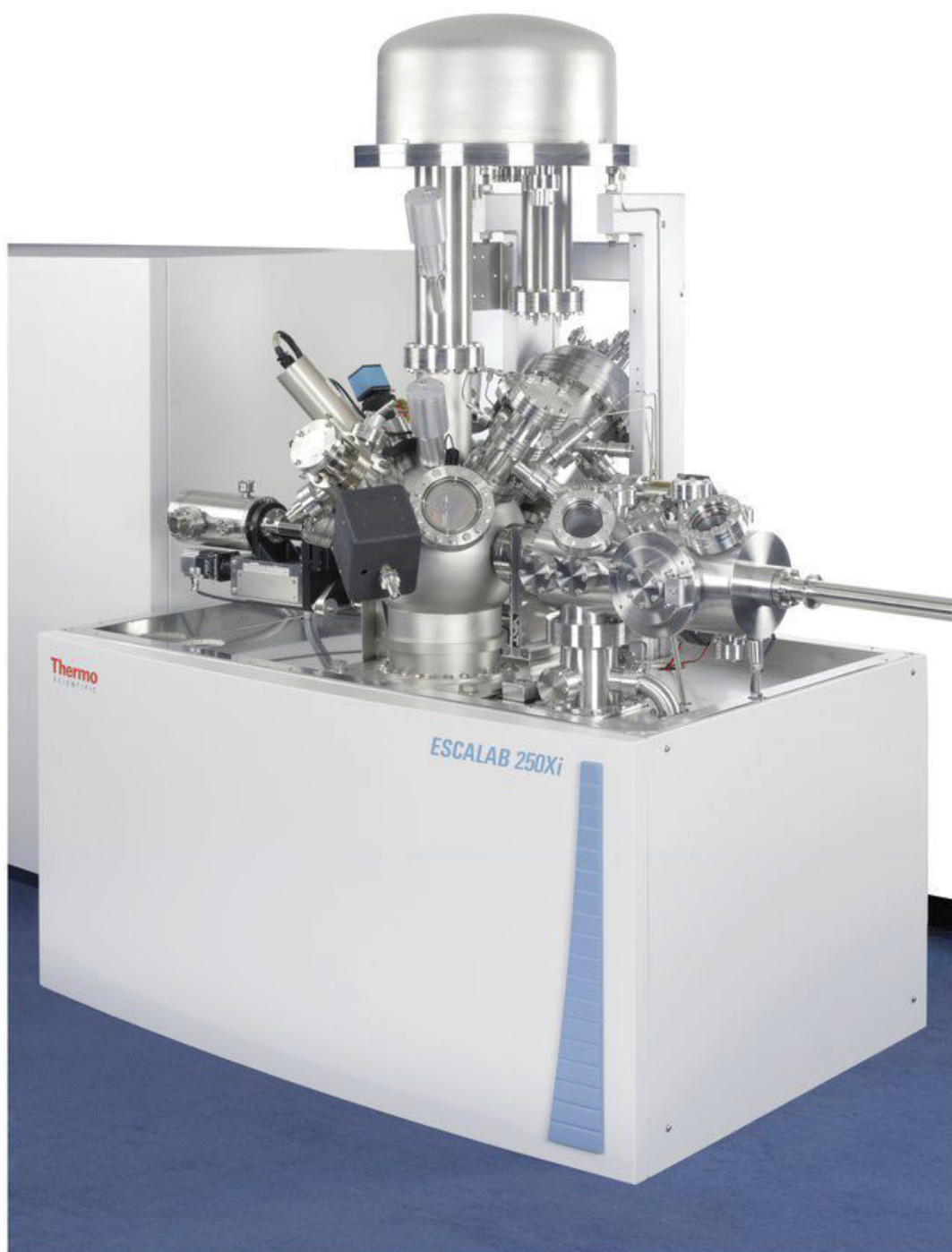
FIGURE 3.7: Thermo Escalab 250Xi spectrometer equipped with an AlK \alpha X-ray monochromatic radiation ( h\nu = 1486.6 eV).©Thermo Scientific - Scientific Instruments and Aut
