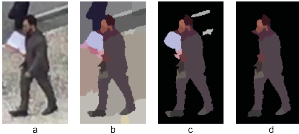
FIGURE 5.6 - EXAMPLE OF DIFFERENT STEPS: a) ORIGINAL (171X91) RGB IMAGE; b) SEGMENTED IMAGE; c) CLASSIFIED IMAGE; d) RESULT IMPROVED BY RELAXATION.
