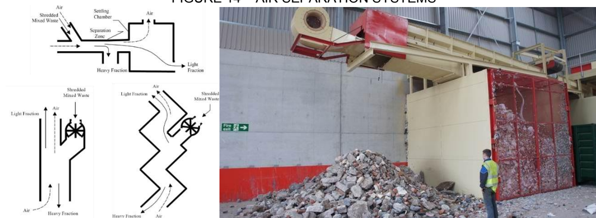
(a) types of air separators, (b) air-knife separator SOURCE: UNEP (2005) and EMS (2019)
