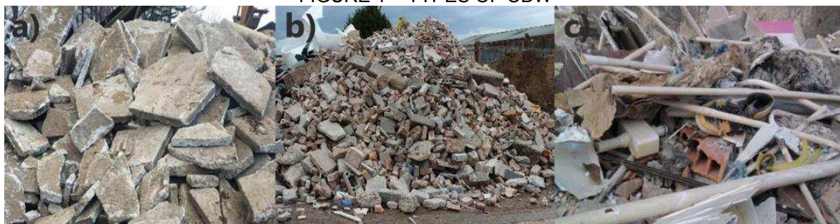
a) mineral CDW, b) "mainly" mineral CDW and c) totally mixed CDW SOURCE: CEG (2017), Nichetti (2019) and Costa (2014)
