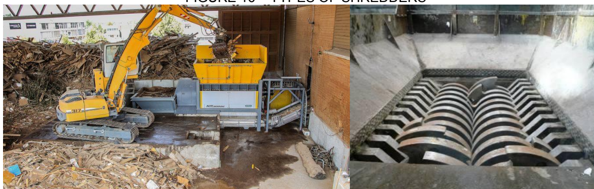
(a) shredder for wood waste, (b) inside a twin-shafted slow-speed shredder SOURCE: WMW (2018) and Wrap (2009)
