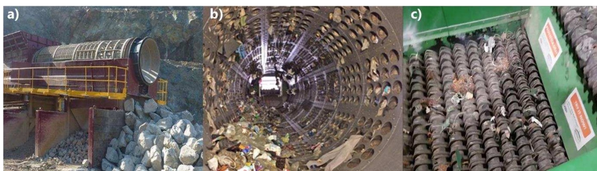
(a) and (b) examples of trommel screen, (c) disc screen SOURCE: BHS (2019), EXCT (2019) and NIHOT (2018)
