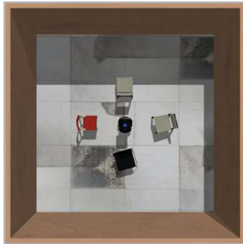
Figura 4.1: Example of a simulation in the Gazebo Simulator from a top view. The robot is at the center, and four different assets are present as obstacles. The scene is a single enclosed room with textured floor and walls with directional light and Phong shading.
