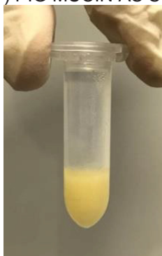
FIGURE 7- 20% (W/V) PIG MUCIN AS SIMULATING SPUTUM
