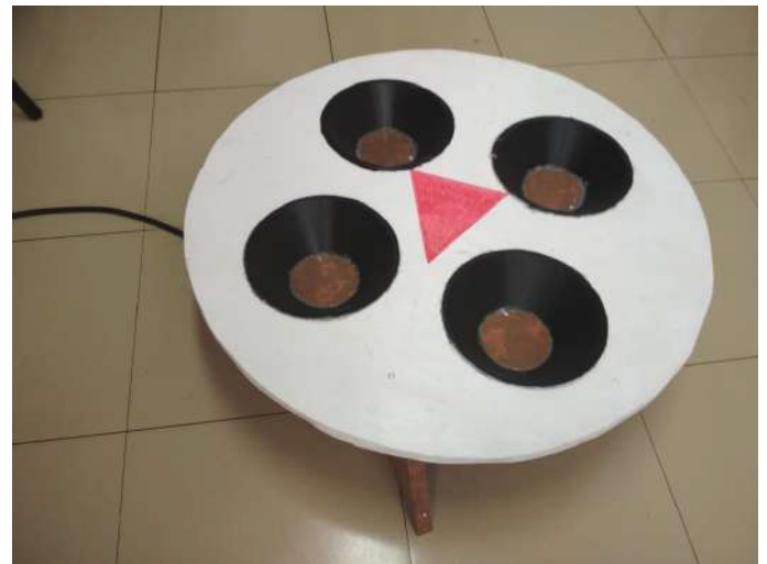
Fig. 5. Prototype of the recharge base developed for landing and recharging of an ArDrone.
