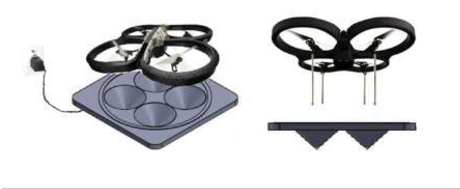
Fig. 3. Representation of the drone approach and contact if the drone feet with metallic contacts at the base.
