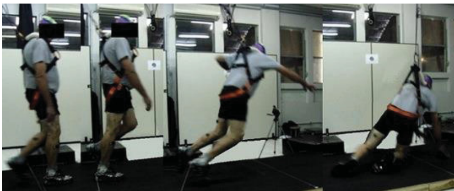
Figure 5.6 – Sequence of images of a participant that was not able to recover balance after the trip. The figure also shows the safety mechanism.
