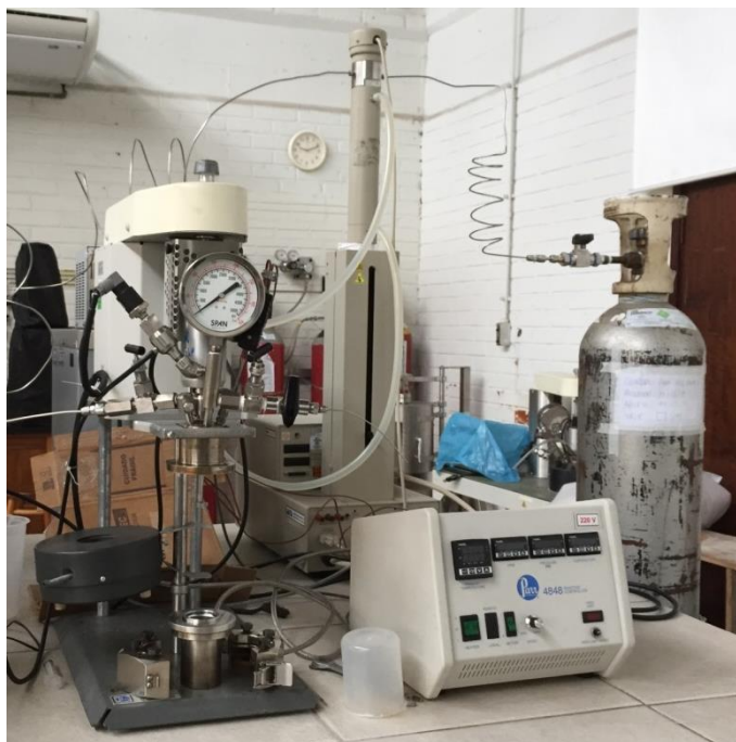
FIGURE 11 – PHOTOGRAPH OF THE CLOSED VESSEL MINI BENCH TOP REACTOR (MODEL 4561, PARR®, USA) EQUIPPED WITH A REACTOR CONTROLLER (MODEL 4848, PARR®, USA).
