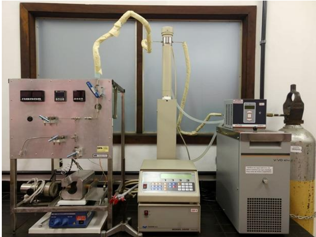
FIGURE 13 – PHOTOGRAPH OF THE EXPERIMENTAL APPARATUS UTILIZED IN THE ESTERIFICATION REACTIONS CONDUCTED IN THE VARIABLE VOLUME REACTOR (VVR) AND IN THE PHASE EQUILIBRIUM EXPERIMENTS.
