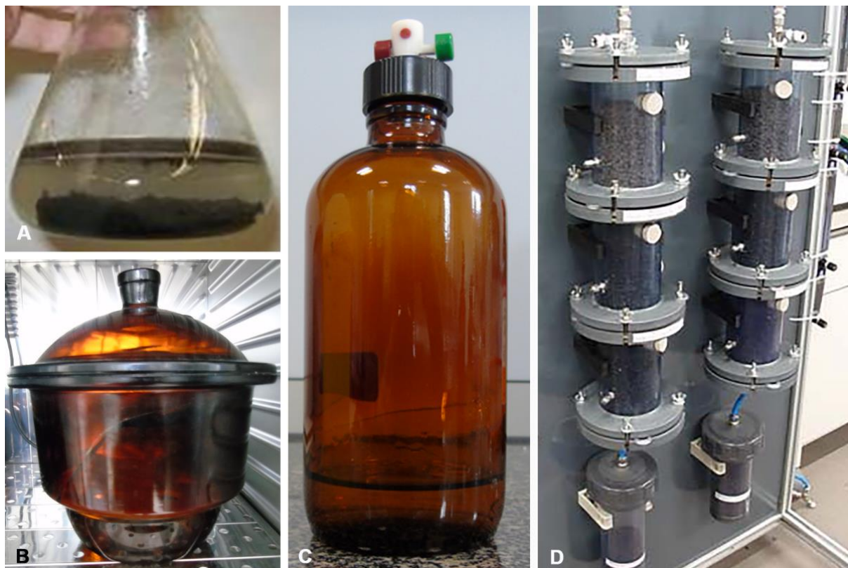
Figure 6 - Selective isolation methods for black yeast-like fungi which degrade monoaromatic hydrocarbon. A – Oil flotation method. B – Solid state-like incubations under controlled atmospheres; C – Liquid batch cultures in sealed vials with Teflon, D – Air biofilter method. Note: A – C: authors personal collection; D: Prenafeta-Boldú, 2013.
