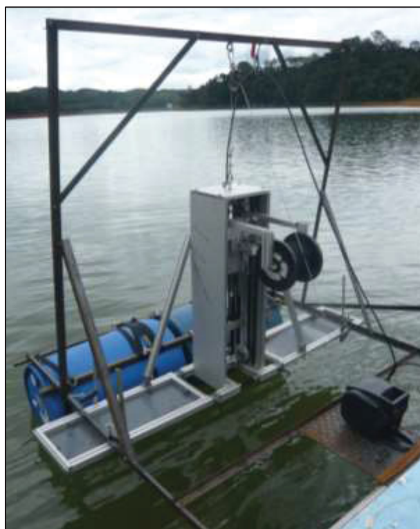
Figure 5-44: The DPS-PS positioned on the floating platform at the side of the vessel in combination with an electric winch.
