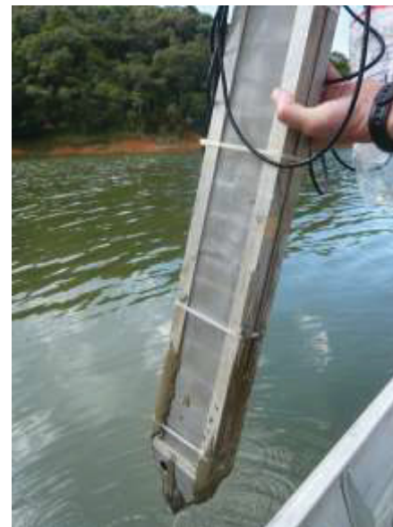
Figure 4-22: DPS after recovery with adherent sediment.
