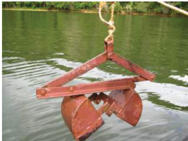
Figure 4-18: Foto of the grab sampler prepared for sampling.
