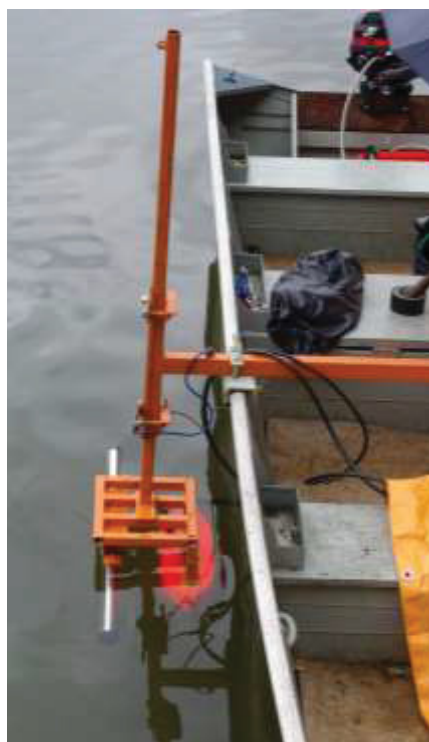
Figure 4-4: The mounted EA 400 echo sounder on the aluminum vessel.
