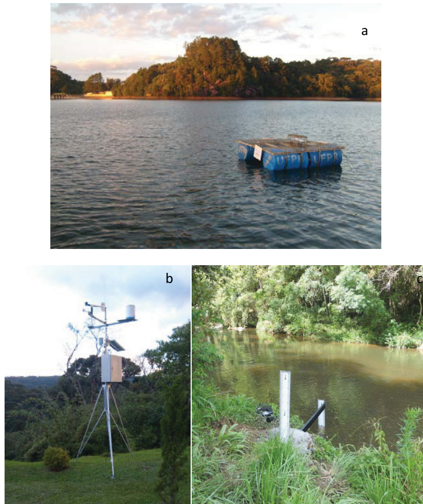
Figure 10 – Vossoroca reservoir monitoring sites a) floating platform and b) meteorological weather station in Vossoroca reservoir and c) Limnometric station in São João river
