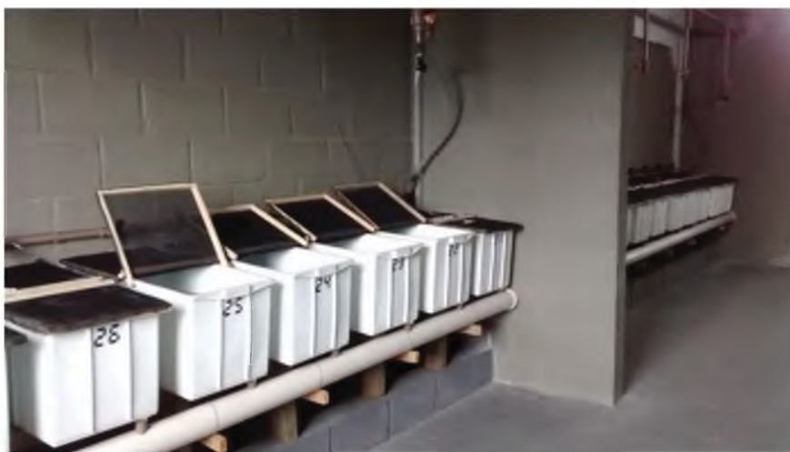
FIGURE 3 Tanks of 50 L capacity and 0.2 m 2 area each, used in the experiment. Photo: S. Amador.
