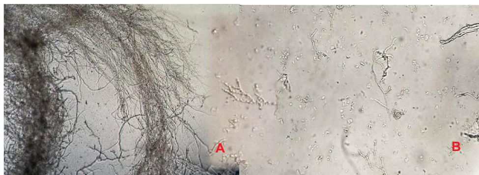
FIGURE 10 – HAND-MIXER DISRUPTION: A) BEFORE MIXING PROCESS, B) AFTER MIXING PROCESS. IMAGES WERE MAGNIFIED 10X.
