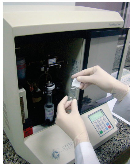
(b) Microscope slide being placed for processing in a Thinprep® 2000 processor. The procedure uses a liquid-based filtration process for slide preparation, whereby the sample is dispersed, randomized, filtered, and a representative sample is transferred to the slide. The automatic process guarantees the thin and uniform distribution of cells.
