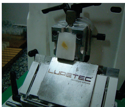
(b) Microtome with trimmed tissue specimen mounted in the paraffin block holder. The block is sliced by the steel blade into extremely thin sections (generally at 1 - 10\mu\text{m} thickness).
