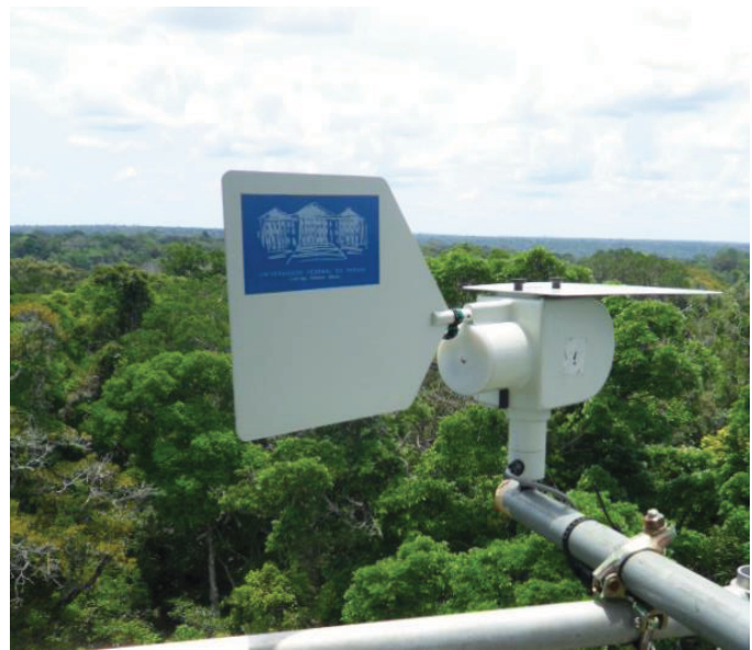
FIGURE 11: The Sporewatch spore sampler: Scheme of the external view describing the parts attached to the main body, with the internal view in detail showing the rotating drum (left), and image of the sampler installed at the tower (right).
