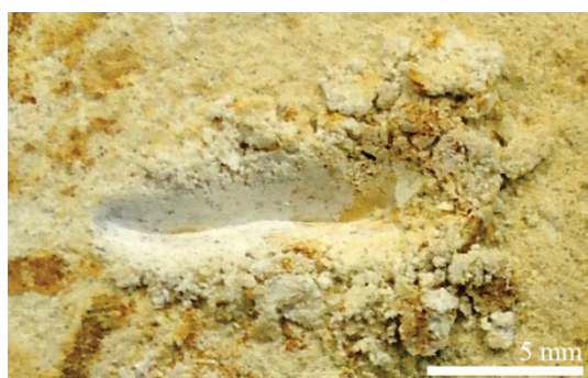
Figure 13 Scratch on sandstone surface with CAI 0.10 display a significant amount of fractured material, deep scratch and a considerable amount of displaced rock material
