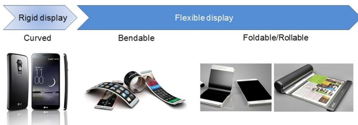
Figure 1.2 Projected trend of the flexible-display technology from a curved device to future flexible devices, such as rollable and foldable displays, that offer many potential advantages, e.g. very thin profiles and lightweight display systems.
