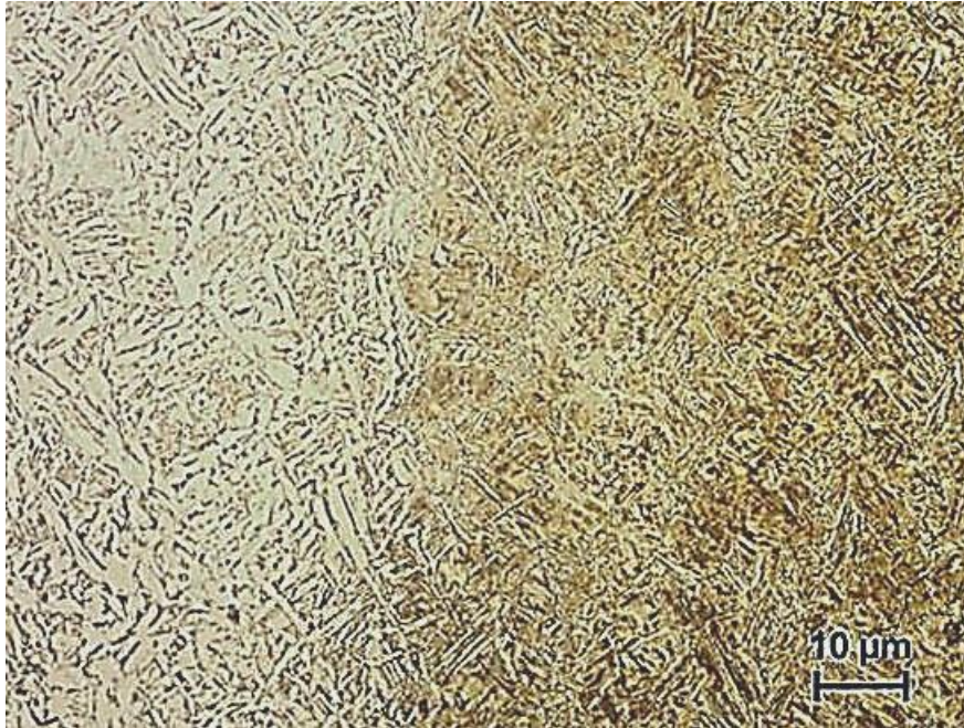
Figura 103. Interface Tubo-Garfo Amostra 3a (Nital 3%, 500x)
