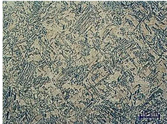
Figura 89. ZTA Tubo Amostra 2 (Nital 3%, 500x) Figura 90. ZTA Garfo Amostra 2 (Nital 3%, 500x)
