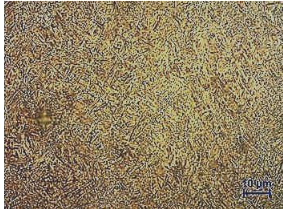
Figura 107. ZTA Tubo Amostra 3b (Nital 3%, 500x) Figura 108. ZTA Garfo Amostra 3b (Nital 3%, 500x)
