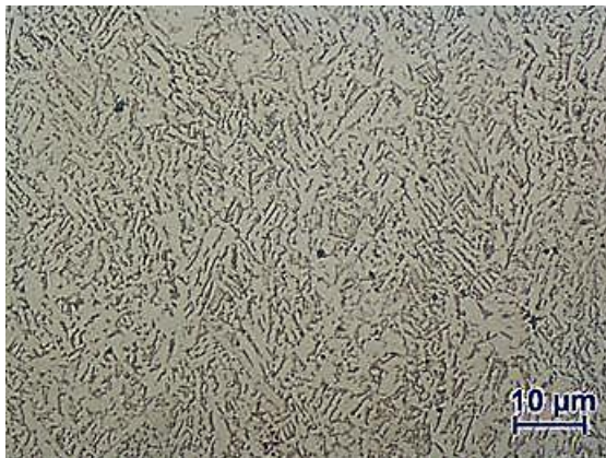
Figura 86. ZTA Tubo Amostra 1c (Nital 3%, 500x) Figura 87. ZTA Garfo Amostra 1c (Nital 3%, 500x)
