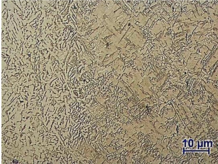
Figura 85. Interface Tubo-Garfo Amostra 1c (Nital 3%, 500x)
