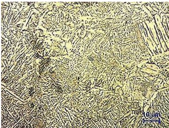
Figura 77. ZTA Tubo Amostra 1 (Nital 3%, 500x) Figura 78. ZTA Garfo Amostra 1 (Nital 3%, 500x)
