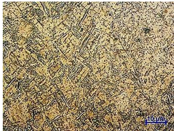
Figura 92. ZTA Tubo Amostra 2a (Nital 3%, 500x) Figura 93. ZTA Garfo Amostra 2a (Nital 3%, 500x)
