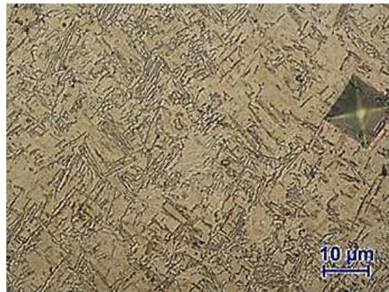
Figura 86. ZTA Tubo Amostra 1c (Nital 3%, 500x) Figura 87. ZTA Garfo Amostra 1c (Nital 3%, 500x)
