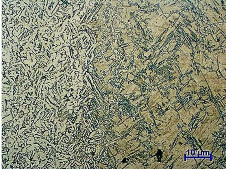
Figura 94. Interface Tubo-Garfo Amostra 2b (Nital 3%, 500x)
