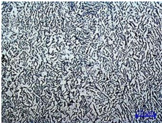
Figura 101. ZTA Tubo Amostra 3 (Nital 3%, 500x) Figura 102. ZTA Garfo Amostra 3 (Nital 3%, 500x)
