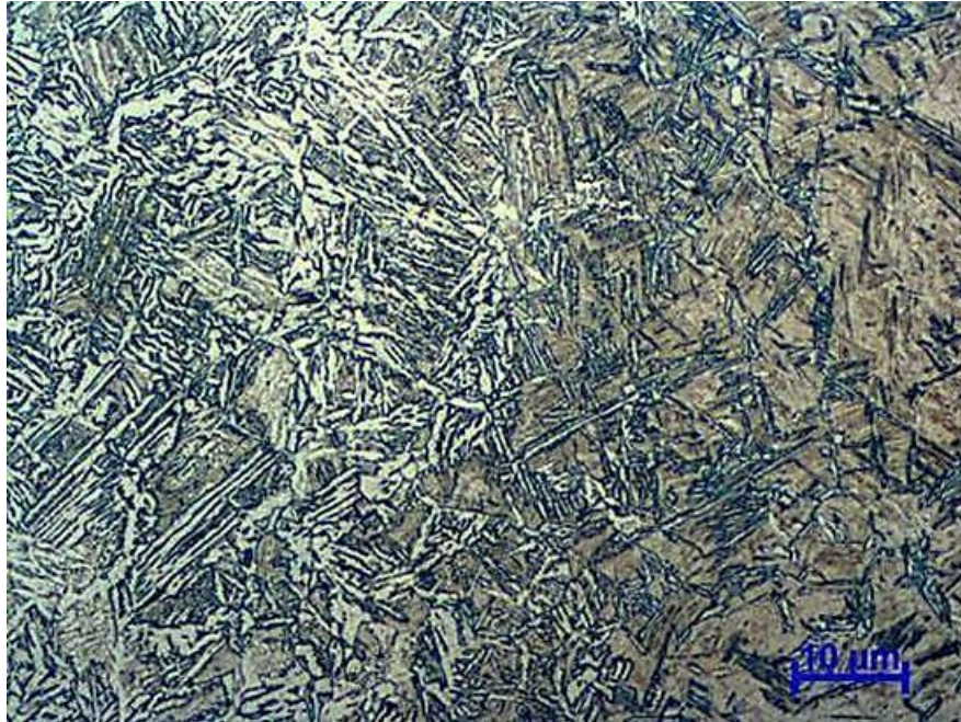
Figura 97. Interface Tubo-Garfo Amostra 2c (Nital 3%, 500x)
