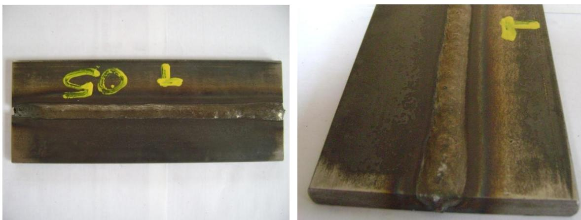
**Figura 4.2 – Chapa soldada com arame tubular 300 A.**
