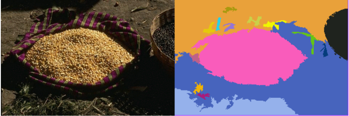
FIGURE 14 – Another example of the Felzenszwalb segmentation. Parameters: \sigma = 0.5 , K = 1000 , min = 100 . From http://cs.brown.edu/~pff/segment/ . Last accessed in 6 Sep 2016.
