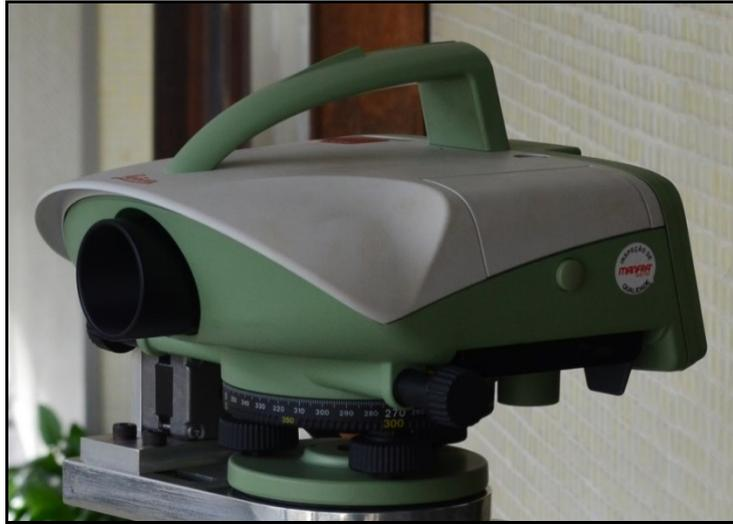
FIGURA 16- NÍVEL DIGITAL DNA 03 LEICA
