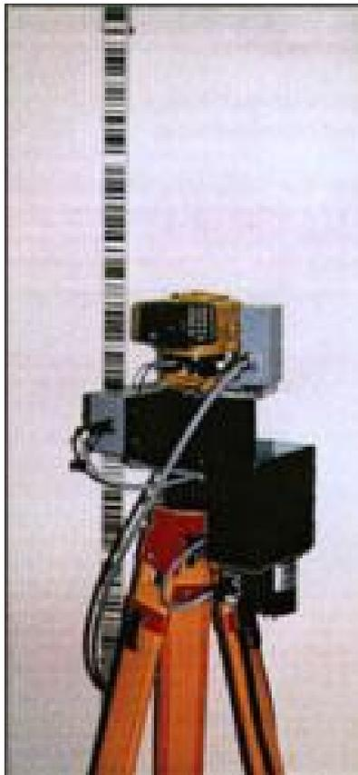
FIGURA 30- SISTEMA DE NÍVEL DIGITAL MOTORIZADO
