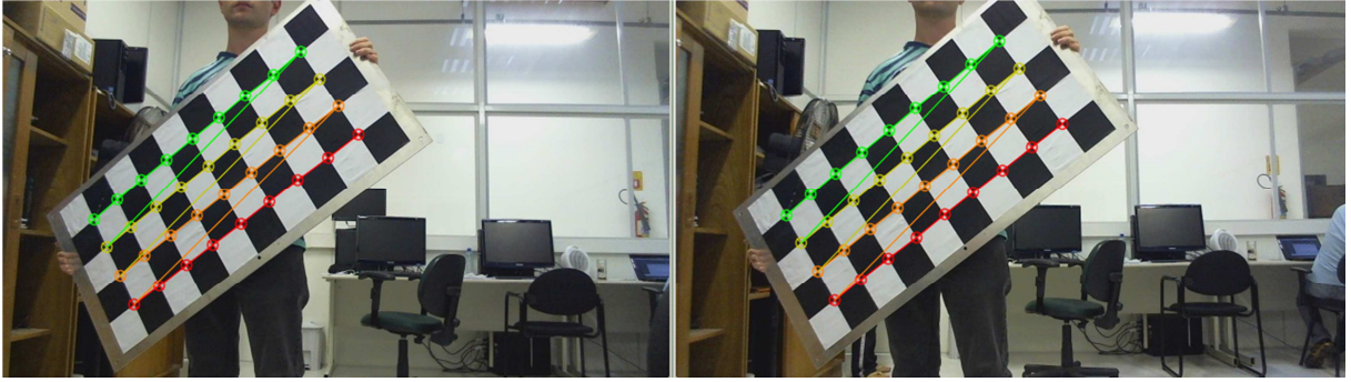
Figure 12: Chessboard pattern being used for calibration aided by the OpenCV library. Overlaid is a pattern showing detected inner corners being used as reference for calibration. (Author's figure).
