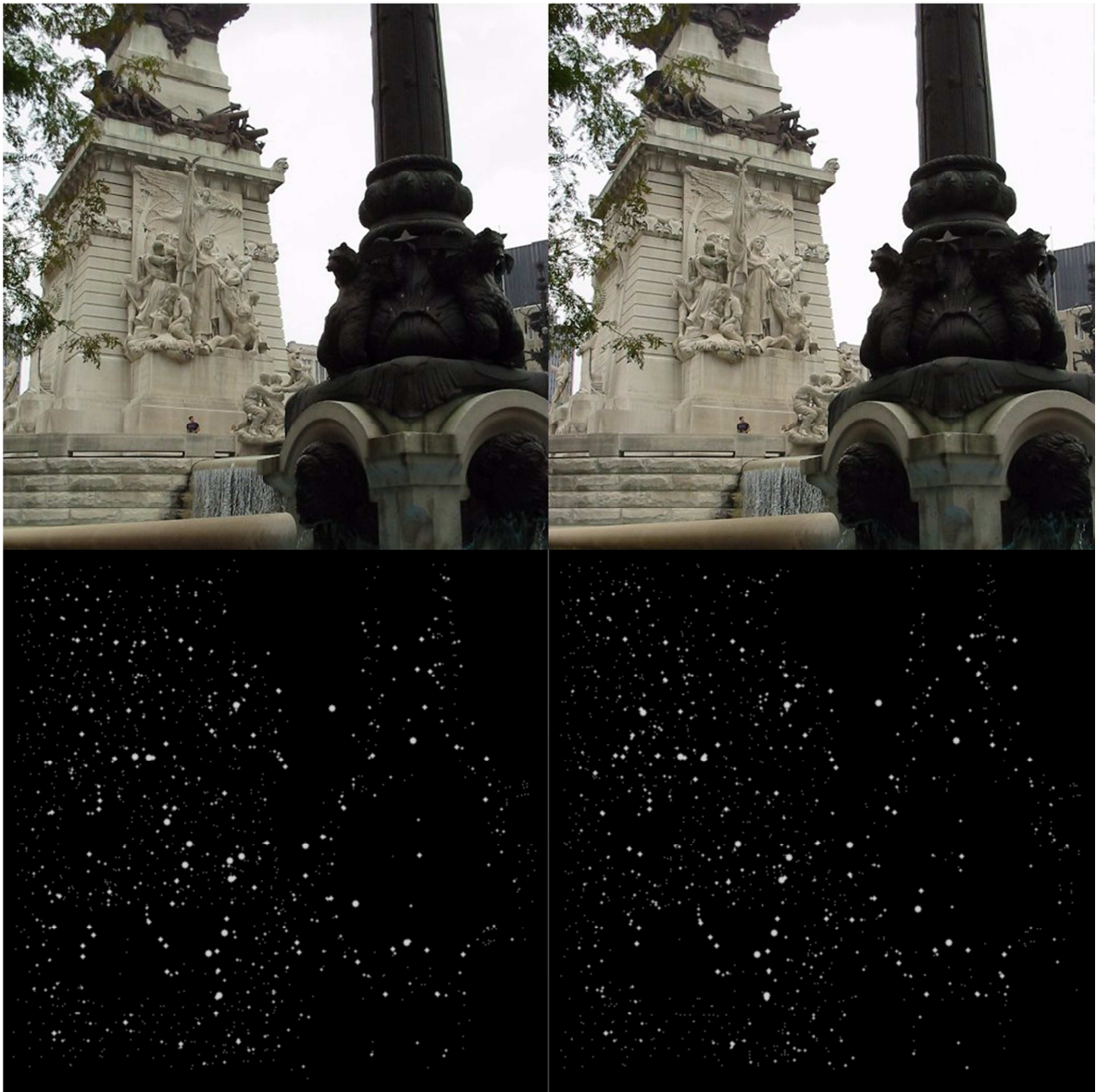
Figure 2: Starry night pattern. POIs detected with SURF are plotted for a pair of image (Callet, 2010) as circles, with radius proportional to the octave of the pyramid where they were detected. (Author's figure).
