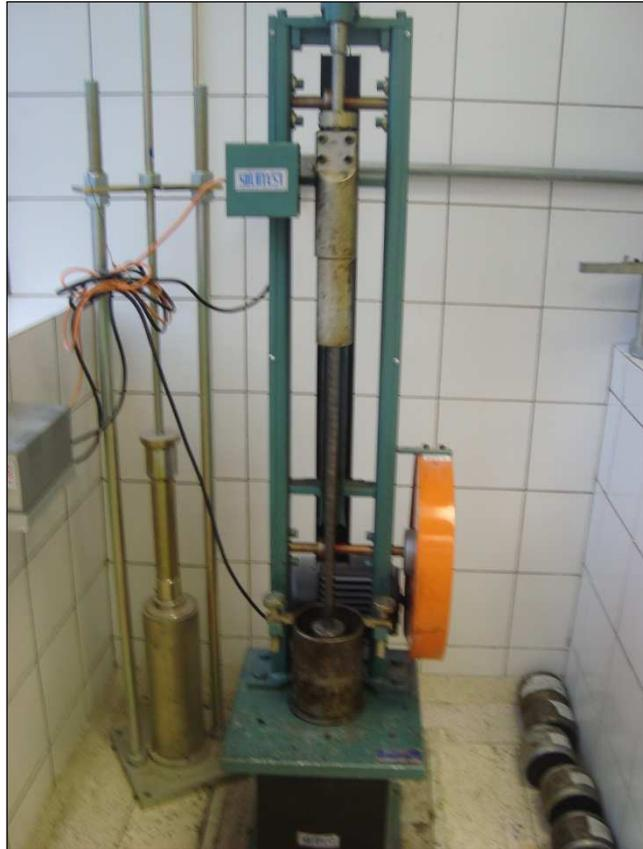
FIGURA 8: COMPACTADOR MARSHALL.
