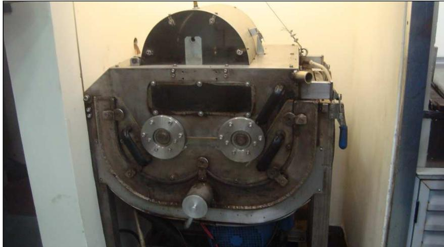
FIGURA 14: MISTURADOR MECÂNICO.
