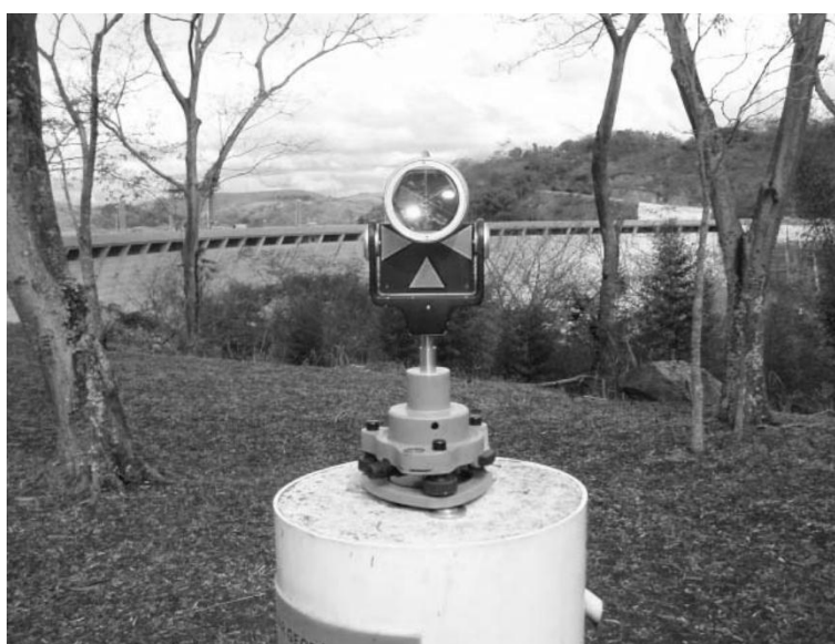
FIGURA 2.4. PRISMA DE MONITORAMENTO - REFERENCE MONUMENT (LEICA GEOSYSTEMS)
