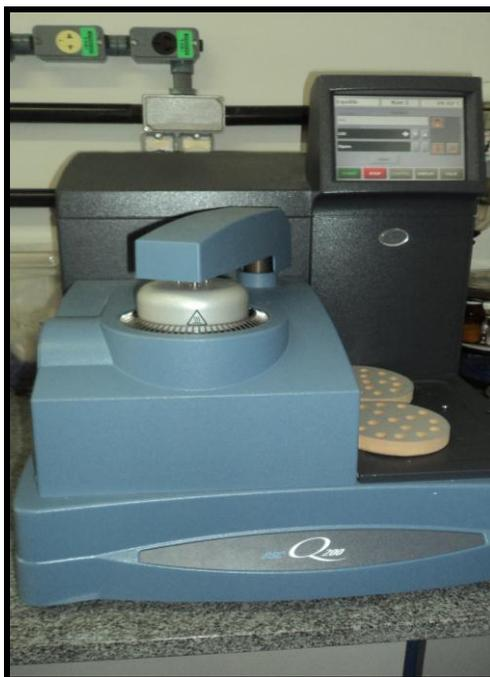
FIGURA 13 – EQUIPAMENTO DE DSC – CALORIMETRIA EXPLORATÓRIA DIFERENCIAL (TA INSTRUMENTS, MODELO: Q200) USADO NAS ANÁLISES (UEPG)
