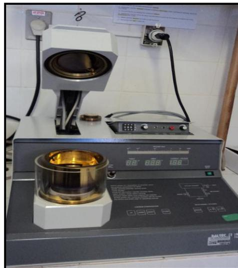
FIGURA 12 – METALIZADOR: BALZERS SPUTTERING SCD-030
